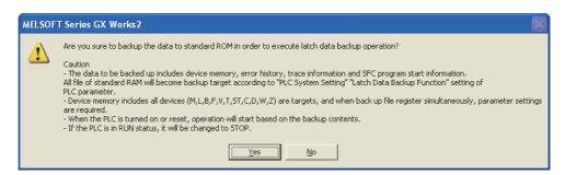
Data to be backed up are the data at the execution of remote operation. After backup, the BAT.LED of the CPU module flashes (green), indicating that the CPU module is in the standby status ready to be powered off.
